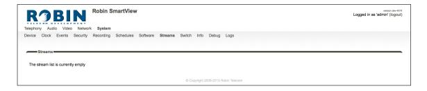
! Note: A maximum of 3 simultaneous video streams are supported. If more than 3 video streams are active, this may adversely affect correct functioning of the intercom. !
